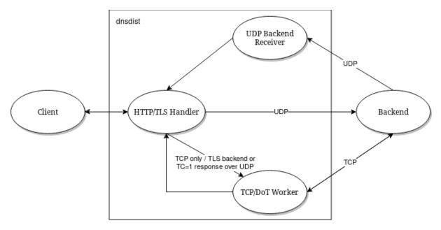
When dealing with a large traffic load, it might happen that the internal pipe used to pass queries between the threads handling the incoming connections and the one getting a response from the backend become full too quickly, degrading performance and causing timeouts. This can be prevented by increasing the size of the internal pipe buffer, via the *internalPipeBufferSize* option of *addDOHLocal()*. Setting a value of *1048576* is known to yield good results on Linux.
