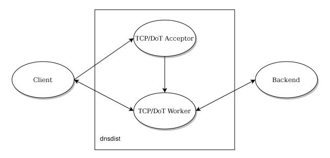
For TCP and DoT, a single thread is created for each *addLocal()* and *addTLSLocal()* directive, listening to the incoming TCP sockets, accepting new connections and distributing them over a pipe to the TCP worker threads. These threads handle both the TCP connection with the client and the one with the backend.
