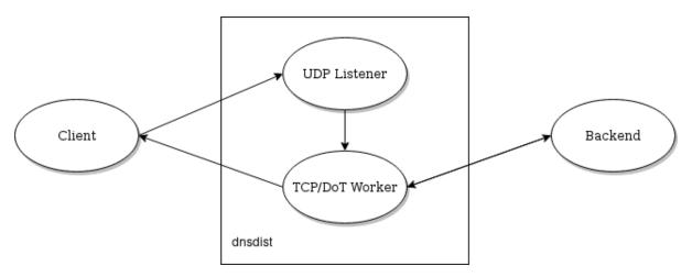
In that case the response will be sent back, directly by the TCP worker, over UDP, instead of being passed back to the UDP responder thread.
