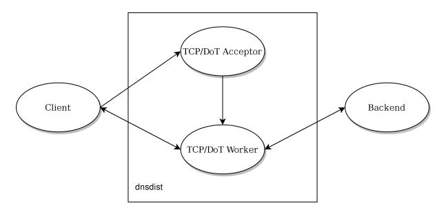
Before 1.4.0, a TCP thread could only handle a single incoming connection at a time. Starting with 1.4.0 the handling of TCP connections is now event-based, so a single TCP worker can handle a large number of TCP
