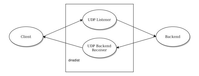
This is great to keep lock contention to a low level, but might not be optimal for setups using a lot of processing power, caused for example by a large number of complicated rules. To be able to use more CPU cores for UDP queries processing, it is possible to use the reusePort parameter of the *addLocal()* and *setLocal()* directives to be able to add several identical local binds to dnsdist:
