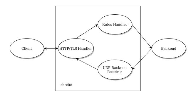
picked up by the regular UDP listener for that backend, the corresponding *IDState* object located, and the response sent to the first thread over a pipe.
